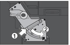
Press the light colored button on the brew unit handle, ①, and turn the handle to the right, ②, to lock it into place.
